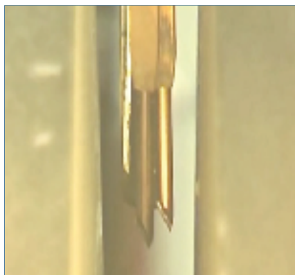
Fig. 3 — Articulating nozzle tips (top) of the AMET narrow groove head showing independent (bottom left) and coordinated (bottom right) wire tip position control.
