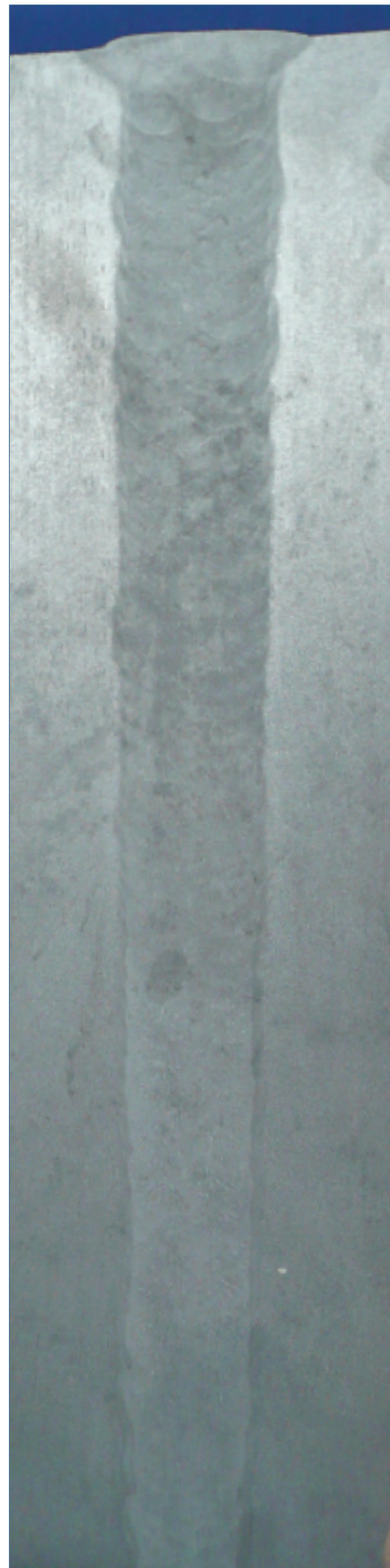
Fig. 1 — Typical narrow groove profile (top left) and cross section of a weld.
