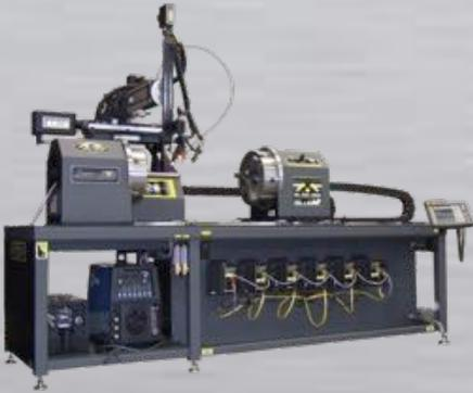
GTAW lathe with AVC, camera system, mechanical oscillation, and synchronized precision headstock and tailstock rotation for creating nuclear industry components.
