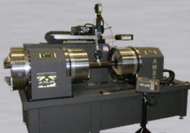
GTAW lathe with dual torch weld heads capable of performing welds at the headstock and tailstock simultaneously. Each weld head has touch retract and AVC capability.
