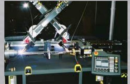
Precision PAW lathe with large pneumatic chucks and synchronized headstock and tailstock rotation for drilling industry components.
