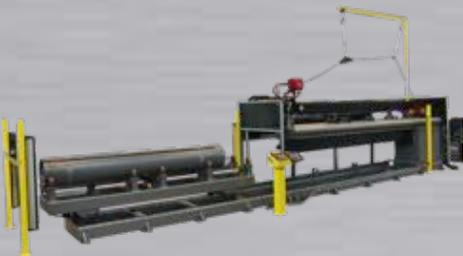
Fully automated GMAW seam welding system for agricultural equipment manufacturing.
