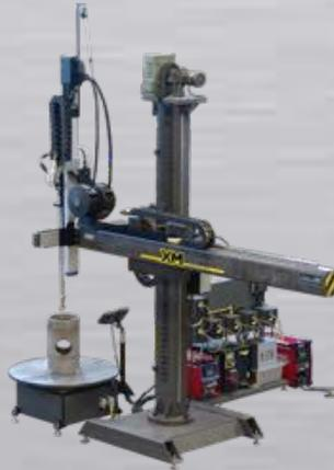
GTAW and GMAW manipulator with separate wire feeders for hotwire GTAW and cold wire GMAW, AVC on both Z and X axes. Includes intersecting bore cladding capability for manufacturing oil and gas industry components.
