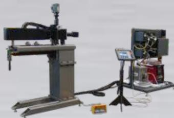
GTAW precision benchtop style seam welder for thin wall stainless steel hose manufacturing.
