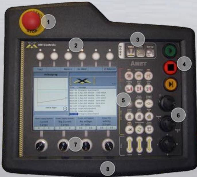
The Start button activates the weld program. The Stop button extinguishes the arc, stops all motion, and advances to the downslope segment of the program. The operator must press the Advance button before proceeding to the next task or weld segment. The Advance feature allows for a pause or a continuous function to be included in the weld program.
