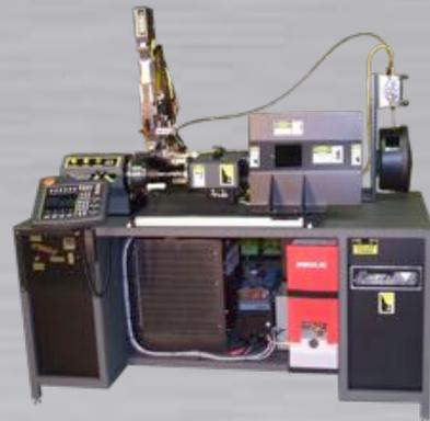
**AMET XM PAW/GTAW Dual Process Precision Benchtop Lathe**
