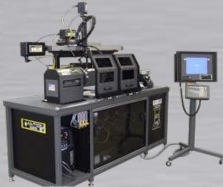
**GTAW Heavy-Duty Bench Lathe with Camera System and Manually Adjustable Weld Screens**
