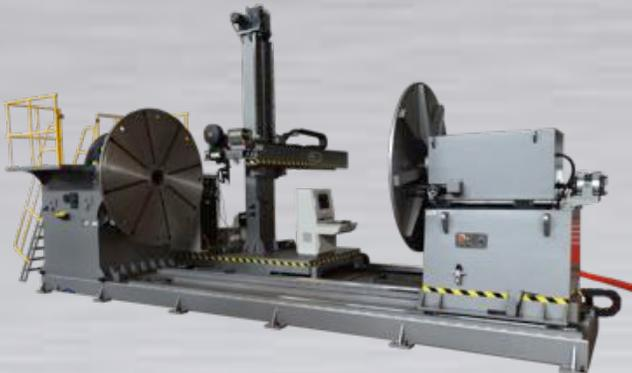
**Large VPGTAW Industrial Weld Lathe with Custom Faceplates and Motorized Tilting Headstock.**
