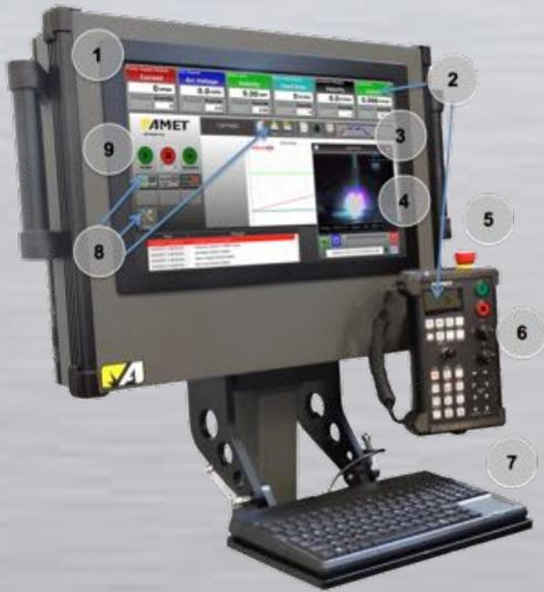
1. The human machine interface includes an LCD touchscreen. The Weld, Edit, and Setup Modes, and their program screens are intuitively presented on the touchscreen for program creation and execution. Simply tap the corresponding area to open the menu, and then use the keyboard for data input.
