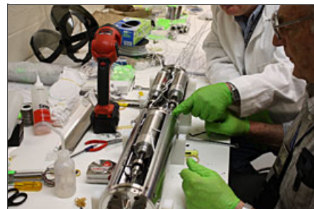
Assembling the inside of the capsule with its various rams, wires and sensors.
