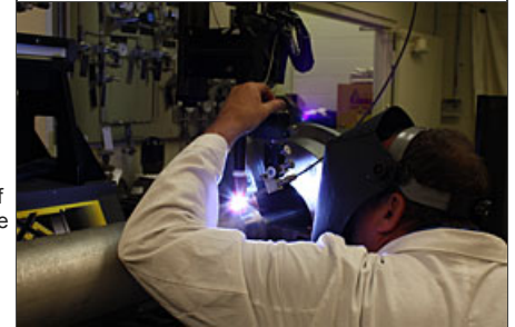
Marv Harker Operates the AMET automatic welder as it joins two sections of the capsule.
