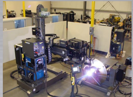
Hotwire GTAW Welding System with Tilting Positioner for Manufacturing On-Board Piping
