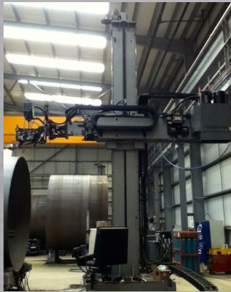
Tandem SAW Windtower Welding System with Telescoping Boom Manipulator
