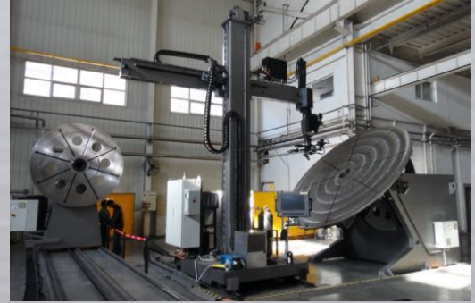
Variable Polarity Arc Welding System With 15 Tonne Tilting Positioner for Aluminum Cryogenic Tank Manufacturing.
