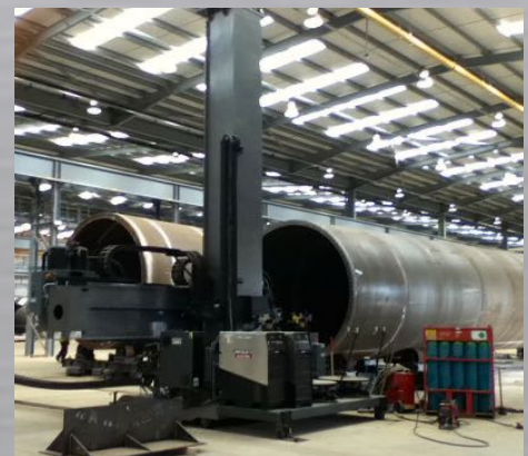
Tandem SAW Windtower Welding System with 90 Tonne Turning Rolls & Fit-up Station
