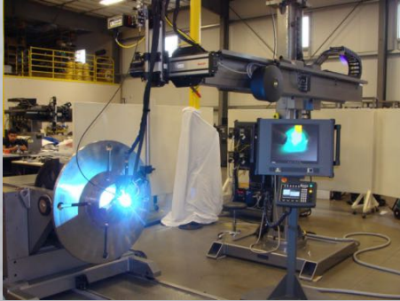
Dab Style GTAW Welding System with Tilting Positioner for Jet Engine Component Repair
