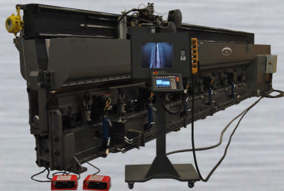
Combination Internal/External dual wire GMAW seam welder for-over-the-road trailer tanker manufacturing.
