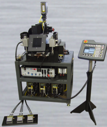
Micro GTA Seam Welder for metal seal manufacturing used in jet engines.
