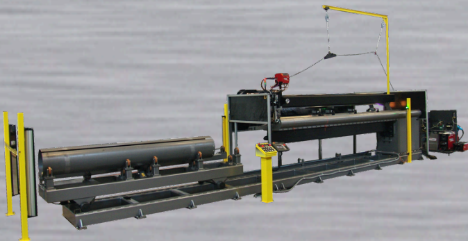
Fully automated GMAW seam welder for heavy agricultural machinery manufacturing
