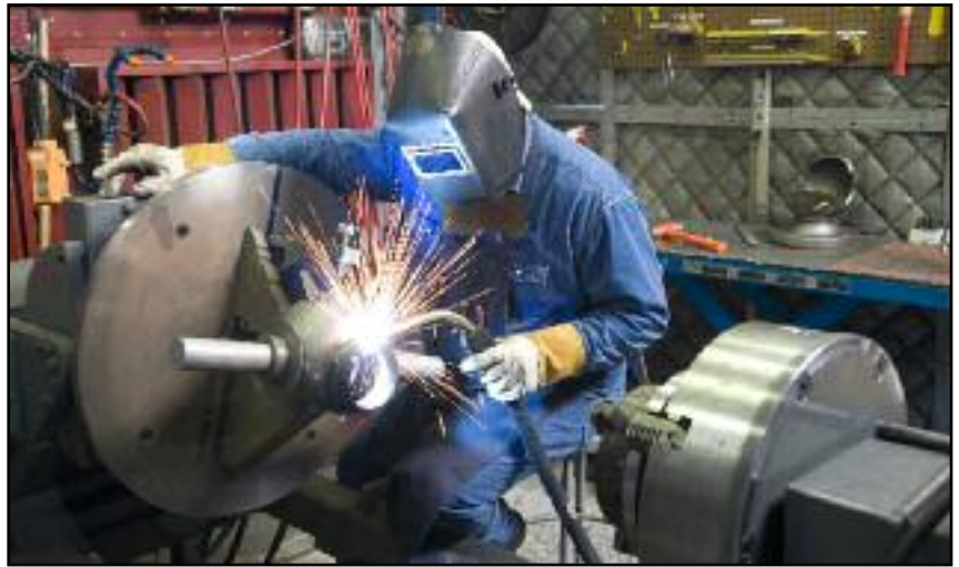
Manual welding of Spherical 3-WAY™ Tee is possible with Lincoln Electric's Power Wave® 455M and Power Feed™ 10M.
