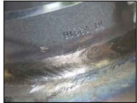
Smooth bead appearance made possible by Lincoln's Waveform Control Technology™ and SuperArc® wire.
