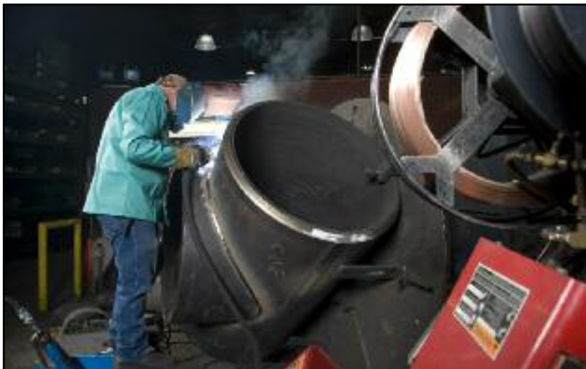
T.D. Williamson welding operators now use a combination of MIG, Submerged Arc and Robotic welding to create many of their pipeline fittings.
