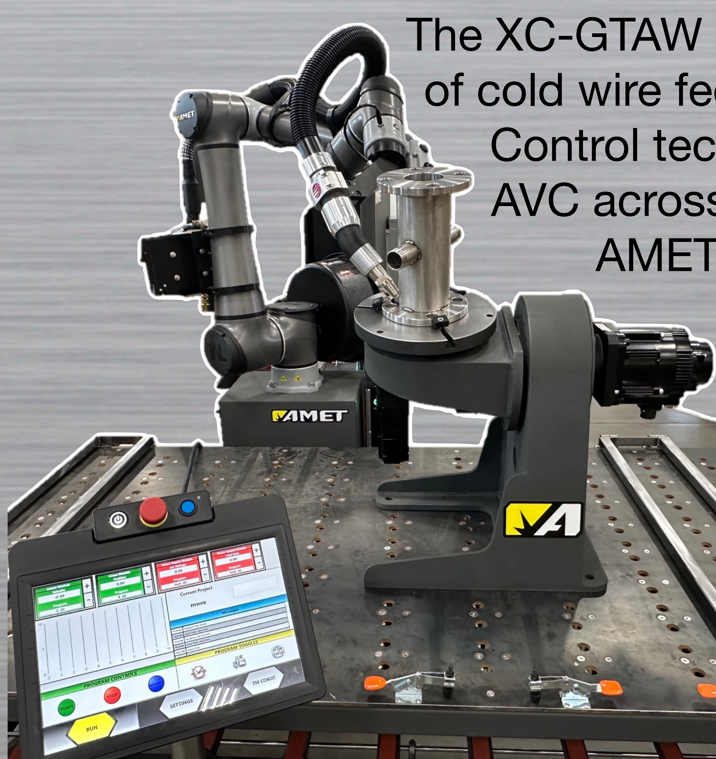
Cobot with integrated tilt and rotate positioner
